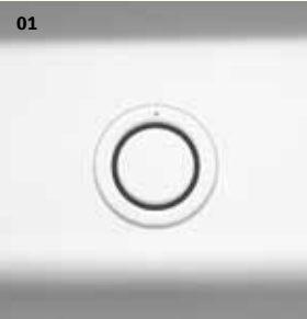
01 Parking aid system sensors The ultrasonic sensors are coloured to match your car's bumper.
