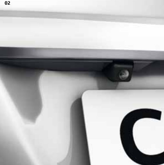
Parking assist The parking assist camera makes reversing even easier by showing what's happening behind your car. You can choose to view the images either on a special rear view mirror or through the screen of your Toyota multi-media navigation system.
